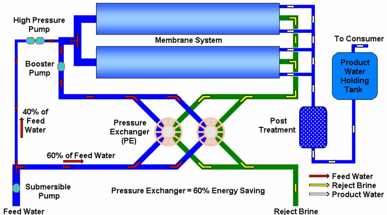
The **Pressure Exchanger (PE)** greatly increases the efficiency of the SWRO system by harnessing the energy of the reject brine. This efficiency can drive energy consumption under 2.8kWh/m<sup>3</sup> of product water. By directly pressurizing a portion of the incoming seawater, the main high-pressure pump size can be reduced by up to 60%. This not only saves energy, it also cuts major capital costs.
